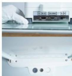
Easy Leveling Simply adjust the feet of the balance until the level indicator shows that the air bubble is centered. This ensures accurate measurements.
